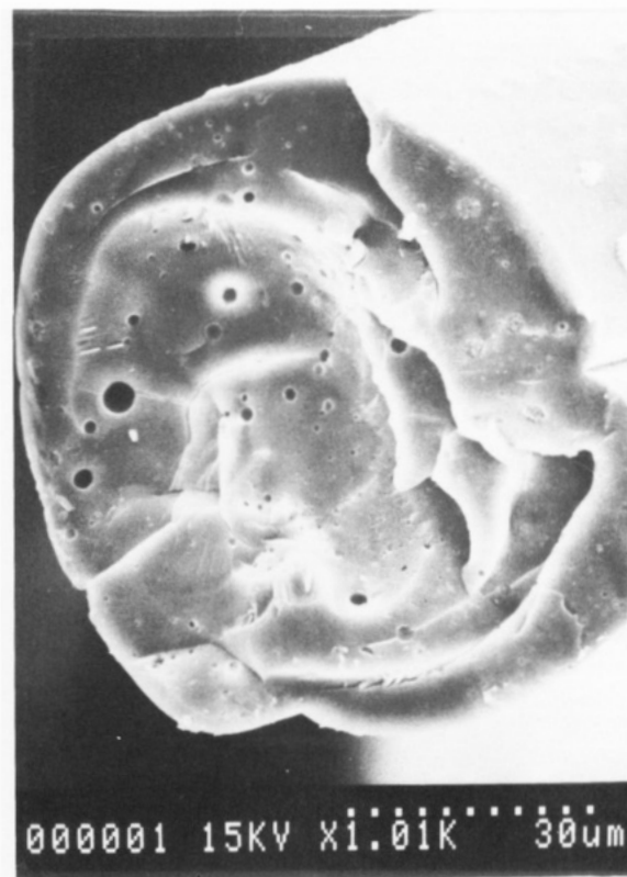
Figure 3. SEM of a fiber end showing cross-sectional detail.
